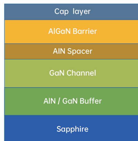
D-Mode Lateral Structure
